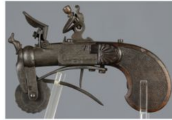
LOT 4348 British Pistol with Henry Nock's Patent Internal Hammer Lock Caliber 60 - Barrel: 9 inch part octagon - Serial Number: NSN - Stock: walnut - Finish: brown. Fitted with Henry Nock's patented internal hammer lock, with London proofed breech, light engravings, silver wire inlays on top of the wrist and a grotesque mask pommel cap. "H.NOCK" marked at the tail of the lock and "crown/GR" Royal cipher at the center. CONDITION: Good overall as refinished, with pitting visible underneath the finish, corrosion, wear, and scratches, dents, repairs and cracks in the stock. Mechanically fine. Estimate:$1,400-$2,250
